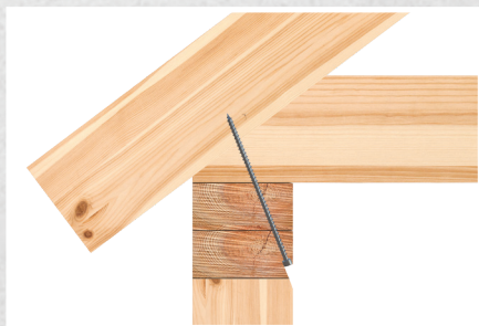
Truss plate removed for clarity.
